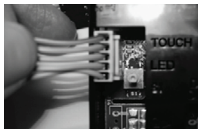
Figure 20 - Connecting end of Touch Pad Cable
