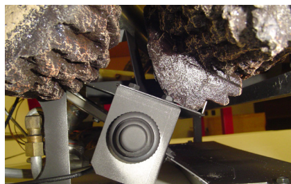
Figure 30A - Installing Front Left Log Side View
