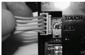
Figure 20 - Connecting end of Touch Pad Cable
