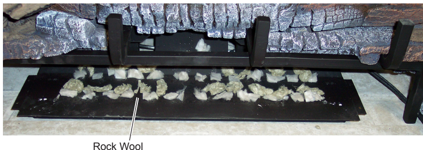
Figure 56 - Placement of Rock Wool (shown with Platinum Bright Embers)
