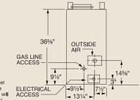
\*If elbows are offset to the back of the unit, chase depth will be 22<sup>5</sup>/8" (575mm).
