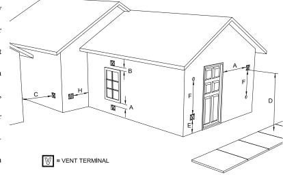
NOTICE: This unit shall be installed in such a way that the exhaust gases are directed so they do not jeopardize people, overheat combustible structures, or enter buildings.
