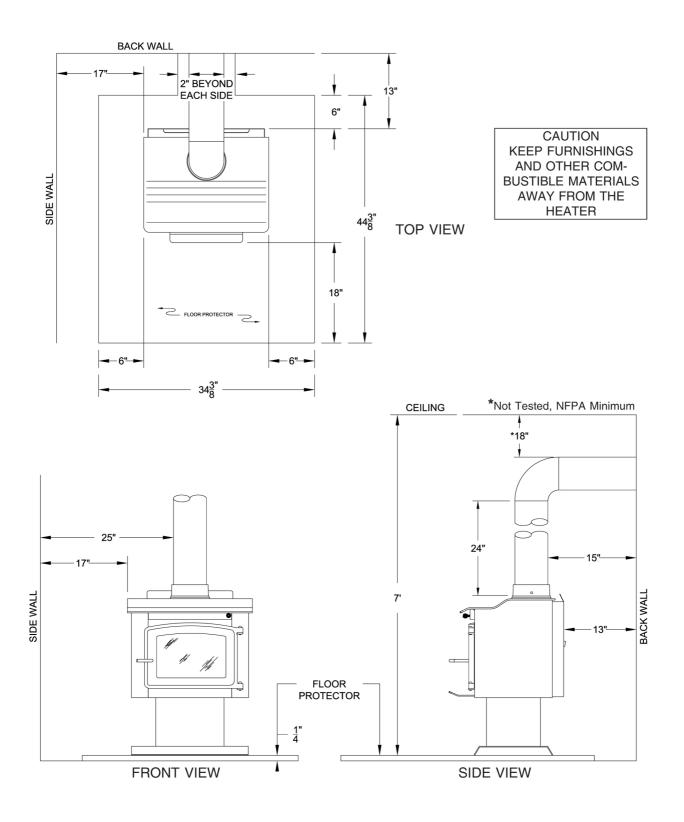
MINIMUM CLEARANCES FOR **CORNER INSTAL- LATION** IS **18 INCHES** FROM THE CORNERS OF THE HEATER TO THE NEAREST WALL
