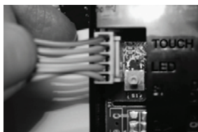
Figure 20 - Connecting end of Touch Pad Cable
