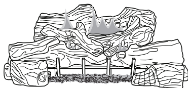
Figure 78 - Correct Middle Burner Flame Pattern
