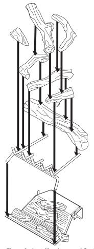
Figure 8 - Installing Logs and Grate
