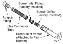
Figure 7 - Venturi Gas Connection
