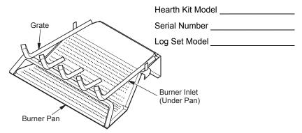
Figure 1 - Product Identification (Ramp Pan Burner)
