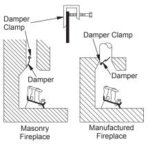
Figure 3 - Attaching Damper Clamp
