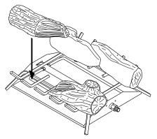
Figure 16 - Placement of Bottom Logs
