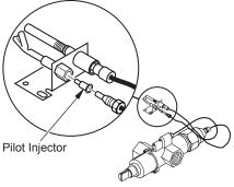
Figure 14 - Installing Propane/LP Pilot Orifice
