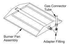
Figure 7 - Connecting Gas to Appliance
