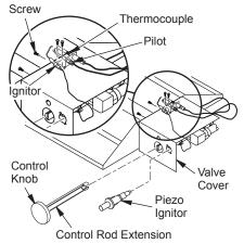
Figure 11 - Installing Cover, Control Knob and Piezo Ignitor
