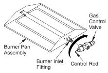
Figure 8 - Installing Gas Control Valve
