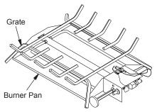
Figure 15 - Installing Grate (Pan Material Not Shown)
