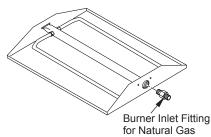
Figure 12 - Remove Burner Inlet Fitting
