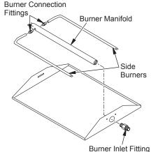
Figure 6 - Installing Burner
