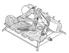
Figure 17 - Placement of Top Logs
